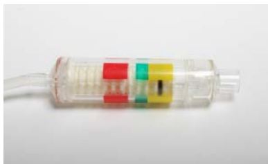
Figure 12: Cuff Pilot Valve in Yellow Zone
